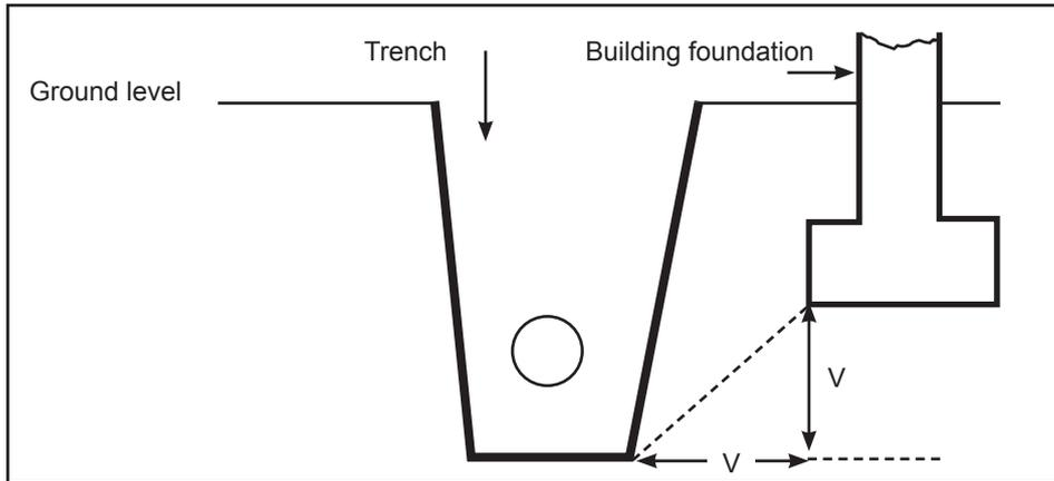
V is equal to the vertical distance between the base of foundation and bottom of trench (2 marks)
