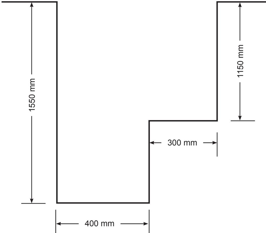
Calculate the volume of material required to fill the trench.
