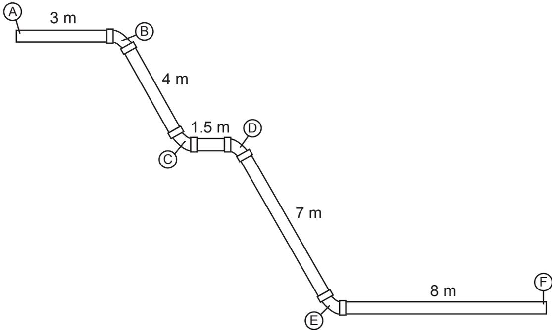
The drain at point F is the sewer connection and is 900 mm below the datum.
