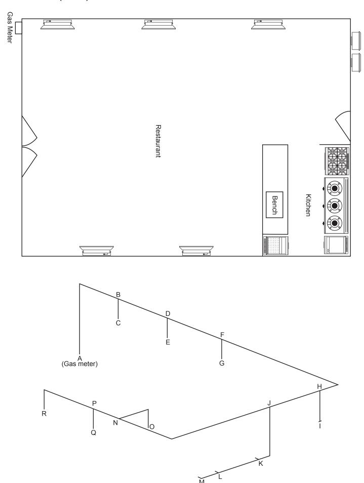
The drawing below shows copper pipework NZS 3501 for a commercial gas installation.
