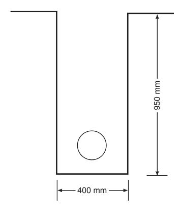
Calculate the volume of material required to fill the trench.
