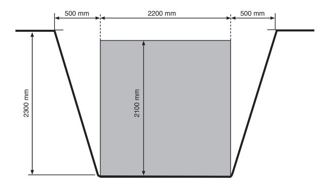
Calculate the volume of backfill material that will be required to fill the trench allowing for 20% compaction.
