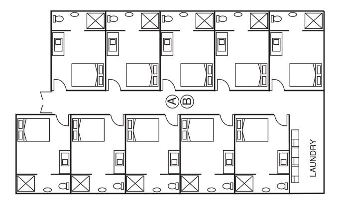
(a) Complete the drawing to show the pipework and components required to convey hot water from the cylinders to the fixtures.
