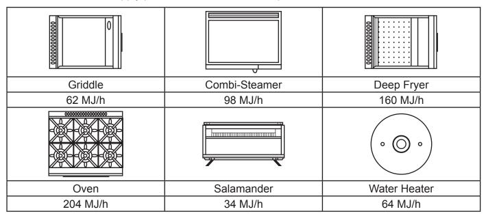
Using the Pipe Sizing Tables from AS/NZS 5601 Part 1 Appendix F starting on page 140, complete the tables below to pipe size the installation. Use the sizing tables and not the sizing graphs to answer this question.
