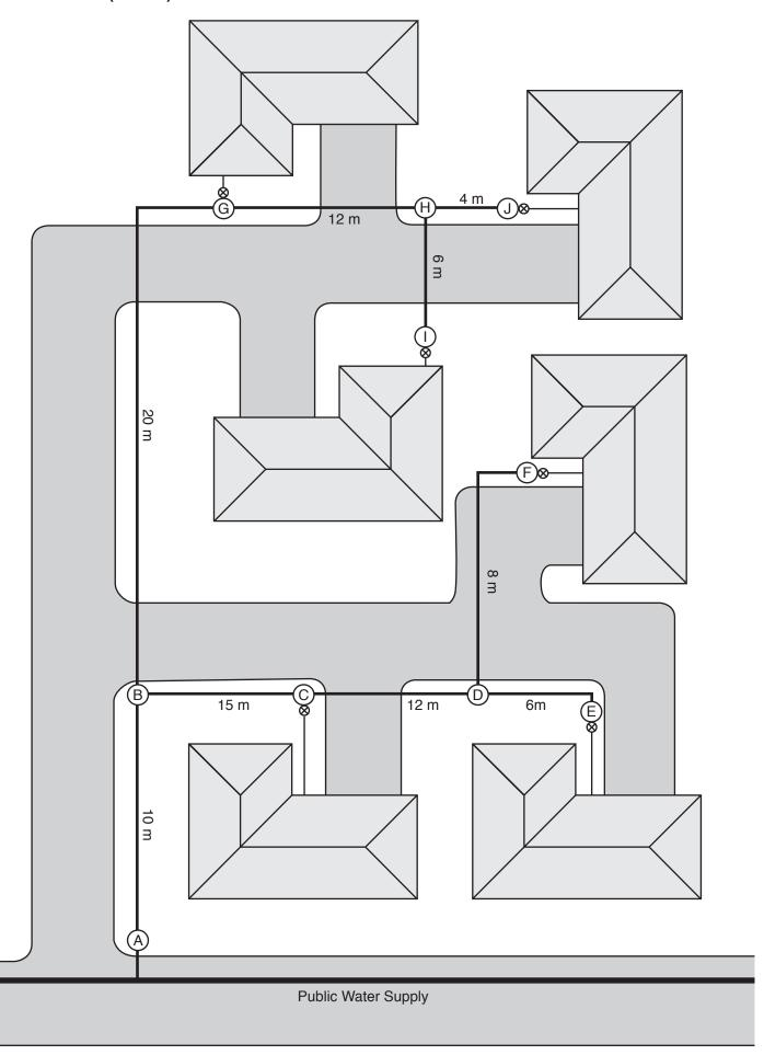
Foul water is to be pumped to a sewer. The pump is capable of reaching 60 kPa pressure.
