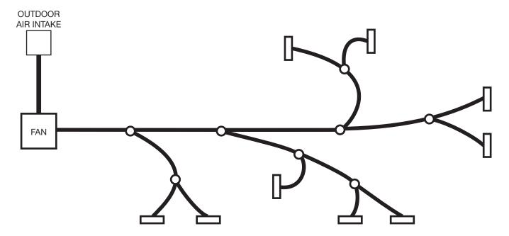
Every section of ducting in the plan is required to be 3 m long.
