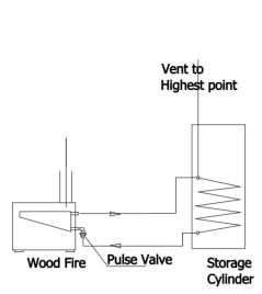
If the cylinder is located below the minimum differential height ( Refer std wetback setup -330 mm) then it is recommended to fit a pulse flow valve.
