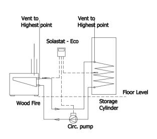
If both connecting pipes are below floor level it is recommended to fit a pump and control thermostat.
