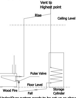
Under/Over system needs to be set up as above with a pulse flow valve to eliminate "back Syphoning"
