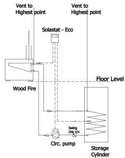
If the storage cylinder is on a lower level than the fire it is recommended to fit a pump and a control thermostat.
